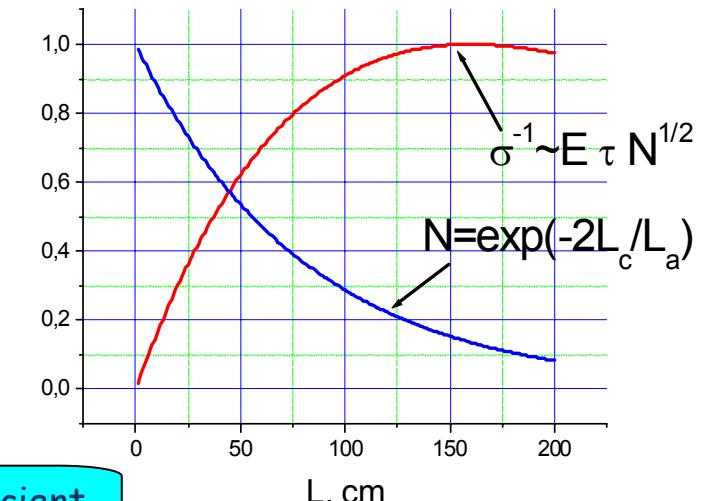
Optimal length of crystal is the two absorption length.
