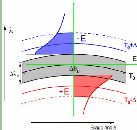
For Bragg angle  $\sim 45^\circ$  the Bragg width  $\sim 0.0005^\circ$
