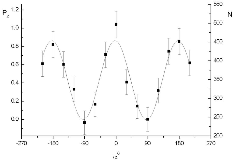
Figure 6: Example of dependence of neutron intensity  $N$  on an angle  $\alpha^\circ$  between Schwinger magnetic field  $\mathbf{H}_g^S$  and vector of polarization of incident neutrons for Bragg angle  $\theta_B = 84^\circ$
