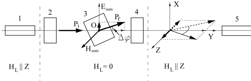
Figure 10: Scheme of the experiment. 1 is a polarizer; 2 is  $\pi/2$  coil around X axis; 3 is  $\alpha$ -quartz monocrystal with sizes  $14 \times 14 \times 3.5 \text{ cm}^3$ ; 4 is  $\pm\pi/2$  coil around Y axis; 5 is an analyzer.  $\mathbf{H}_L$  is a guiding magnetic field;  $O \parallel Z$  is an axis of a crystal rotation;  $\mathbf{P}_i$  and  $\mathbf{P}_f$  are the polarization of neutron beam before and after the crystal correspondingly
