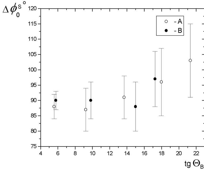
Figure 7: The dependence of an angle of neutron spin rotation due to Schwinger interaction  $\Delta\phi_0^S$  on the tangent of Bragg angle. **A** and **B** – two crystal positions (see Fig. 1 and Fig. 2)
