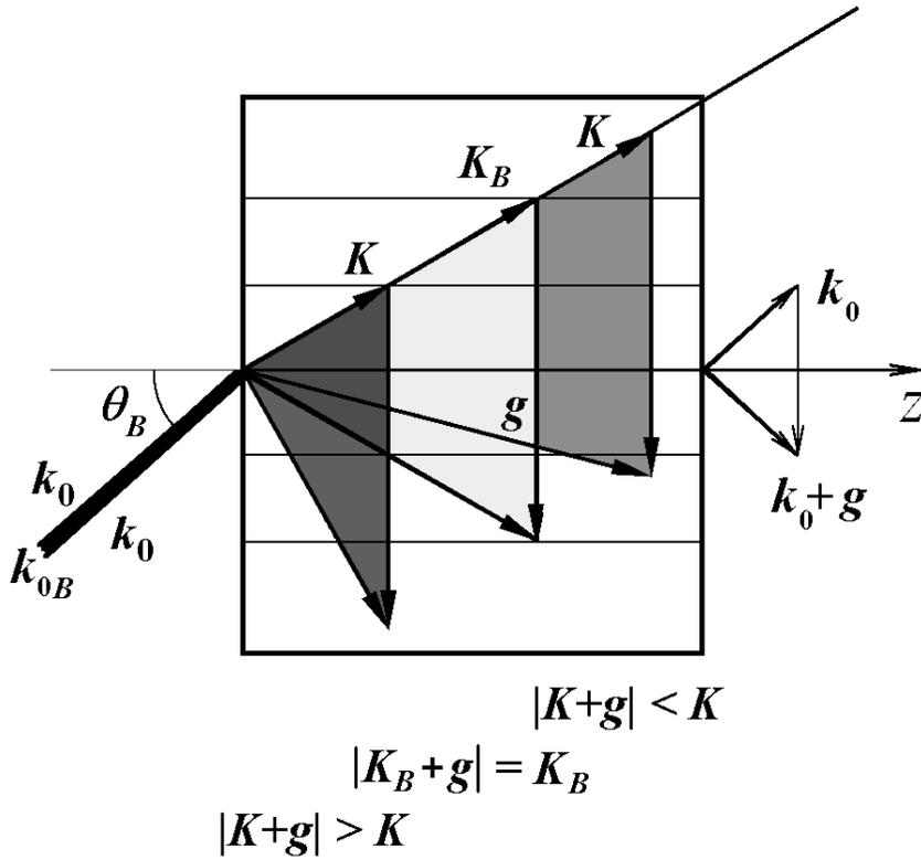
Figure 9: Scheme of the neutron movement in the crystal with the wave vectors  $\mathbf{K}$  of given direction but of different absolute values (different wave lengths). The same three cases as in the Fig. 8  $|\mathbf{K} + \mathbf{g}| > K$ ,  $|\mathbf{K} + \mathbf{g}| < K$  and  $|\mathbf{K} + \mathbf{g}| = K$
