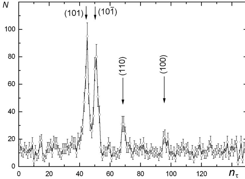
Figure 3: TOF spectrum of the direct diffracted neutrons for Bragg angle  $\theta_B = 75^\circ$ .  $n_\tau$  is the order number of the TOF channel. The width of the TOF channel is equal  $\simeq 51.2 \mu\text{s}$ .  $N$  is the number of accumulated events
