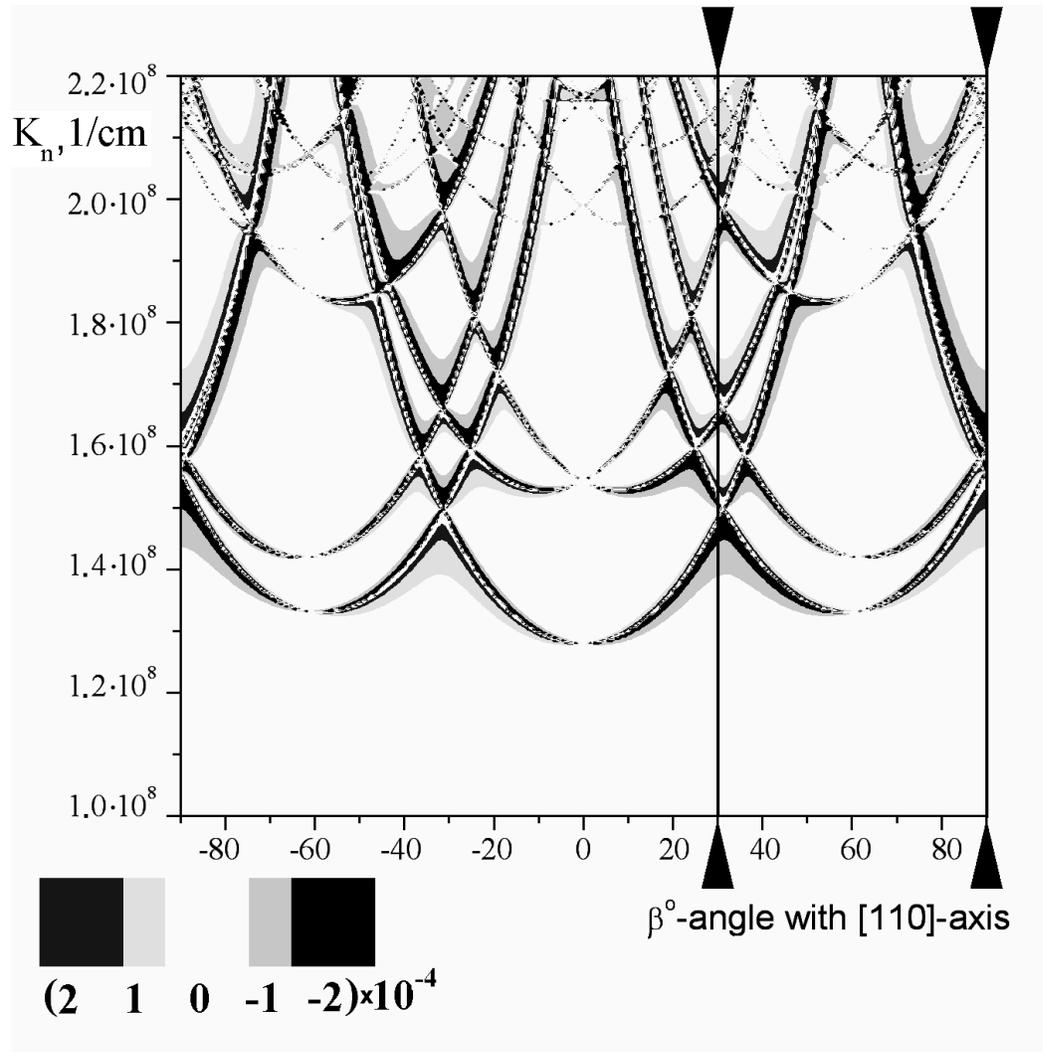
Figure 12: Theoretical dependence of  $\Delta\varphi$  on the wavevector and direction of neutron for the  $\alpha$ -quartz crystal (see Fig. 2)
