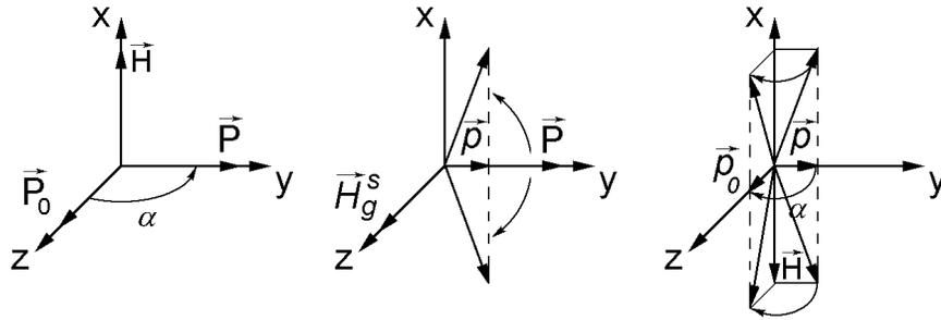
Figure 5: The behaviour of the diffracted neutron spin for the case  $\alpha = 90^\circ$
